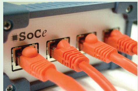
**PROFINET*Switch*** can be used in combination with **SoCe HSR-PRP*Switch*** IP to introduce HSR and PRP capabilities in the ports that were required.
