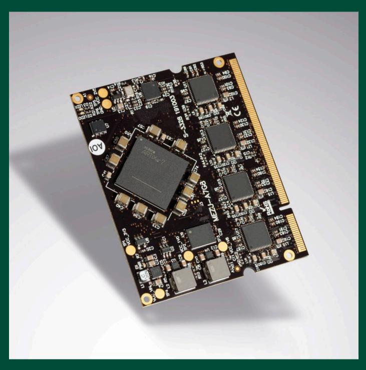
Up to 8x 1GbE ports pluggable module with SO-DIMM format
