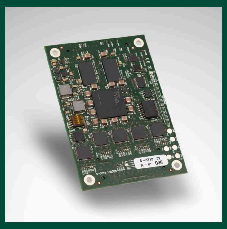
Up to 5x 1GbE ports pluggable module with reconfigurable networking capabilities
