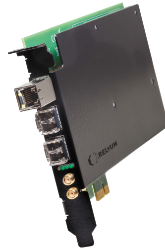
Figure 3 RELY-SYNC-HSR/PRP-PCIe card plugged on the PC Server.
